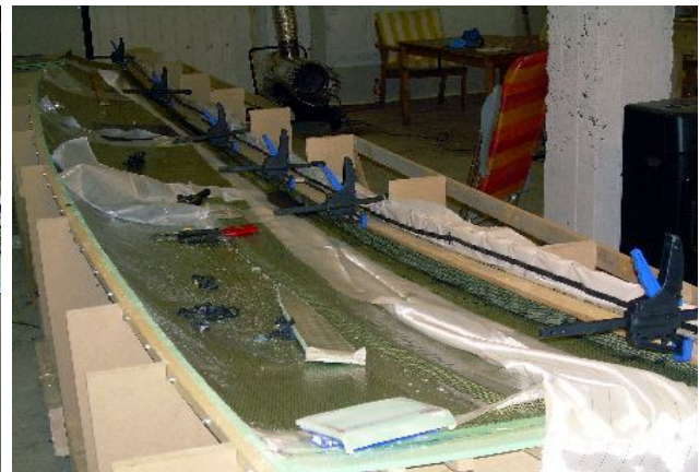
Laying up the deck flange by hand, lots of dirty work and 2nd grade result. I will lay down one layer before infusion next time, to use as an air tight form.
