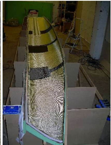
All layers in place except the deck flange
