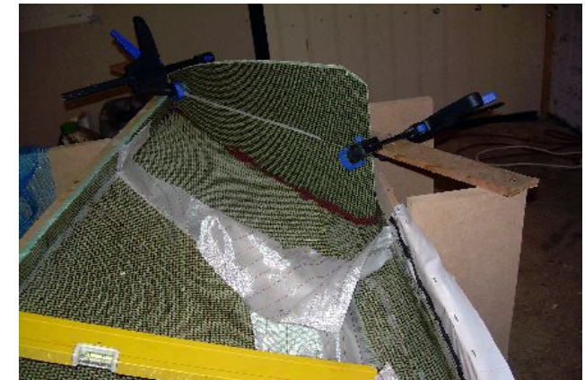
Laying up the deck flange by hand, lots of dirty work and 2nd grade result. I will lay down one layer before infusion next time, to use as an air tight form.
