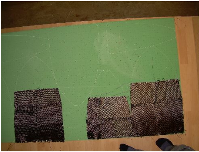
Laying up for infusion of bulkheads, first the reinforcements
