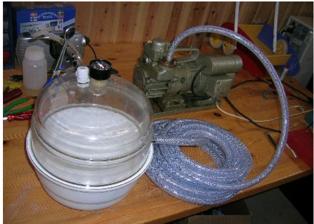
Overflow chamber with removable bucket and pressure gauge
