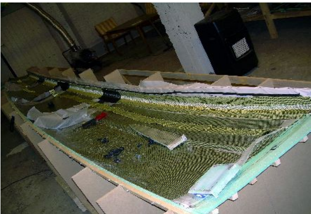
Laying up the deck flange by hand, lots of dirty work and 2nd grade result. I will lay down one layer before infusion next time, to use as an air tight form.
