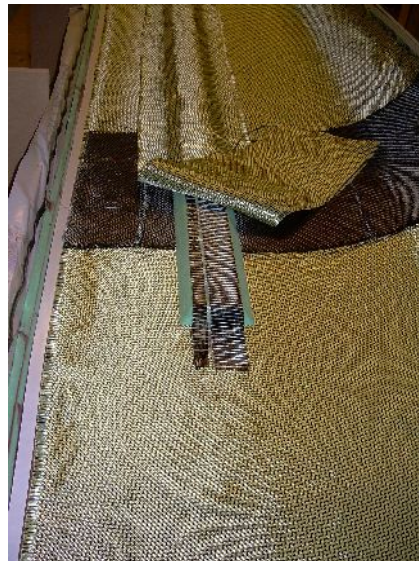
Reinforcements and bow stringer with UD carbon
