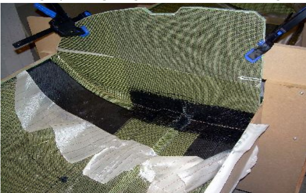
Laminating bulkheads and vacuum bagging the shroud backing plate
