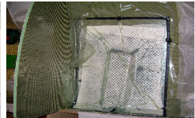
Laminating bulkheads and vacuum bagging the shroud backing plate
