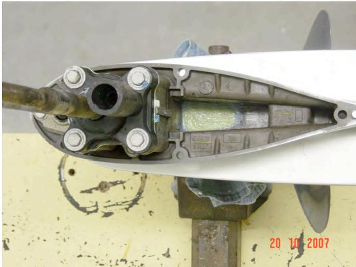
Step 1 Remove the lower leg by disconnecting the gear change rod and removing the five bolts. Carve a bit of structural foam to the shape of the exhaust channel, smear it with silicon, and jam it into the hole level with the cav plate. Obviously clean the metal surfaces first. The green Airex is visible in photo. I used Klegecell in the Evinrude, and it was still there after 11 years.
