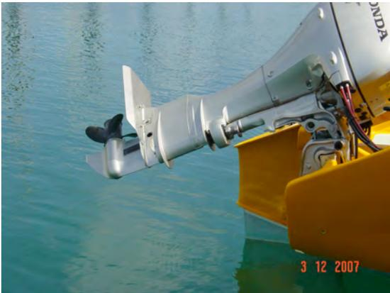
Step 3 Depending on your brand of outboard, immersion depth, and where it is safe to locate the exhaust holes, test and see if you need a cav plate extension. (Of course, you remembered to make a cardboard template before you relaunched just in case you needed to make the plate.) Don't spend over \$100 on a commercial one, as they are designed for a planing situation, sit too far back for this problem, and are too wide so foul your rudder blade – F32 anyway.
