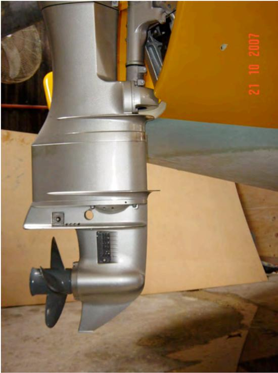
Step 2 Drill 1” holes on each side of the leg above the cav plate. Make sure you are not cutting through any structural webs, only plain wall section. Replace leg.
