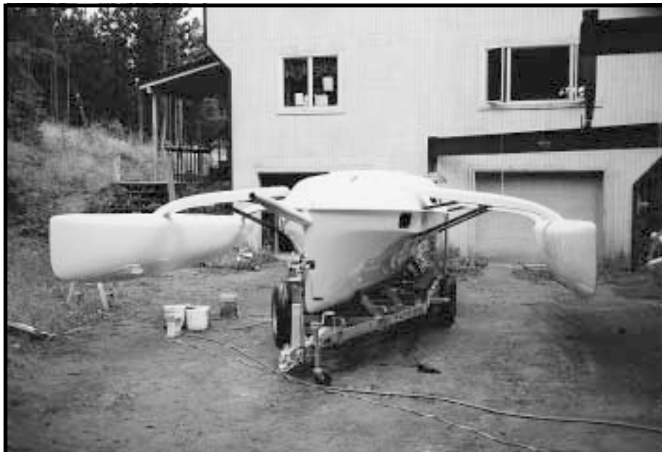
Another New F-25C Bill and Leslie Adam's F-25C nearing completion in Colorado, with a superb paint job. Bill and Leslie own Colorado Composites, who build the high tech. F-25C hulls for MPG Marine. Note the opening window ports on the side of main hull bow for very effective ventilation of the fwd. bunk, while improving forward visibility - they are also rain proof, being located under join flange.
