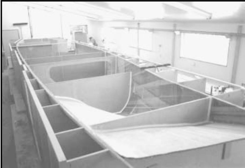
*Scott Webster's first F-36 main hull port half, near completion. Cedar strips are being used above gunwale for wood appearance, foam strips below for lightness*
