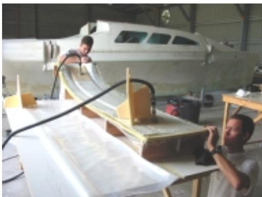
*Beam tops being vacuum bagged*
