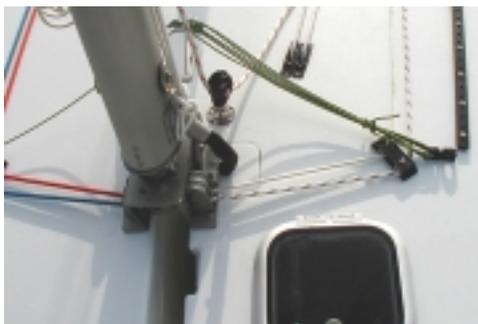
**Deck recess with flush cover for mast electric/VHF plugs**, to keep them below deck and away from feet/damage.
