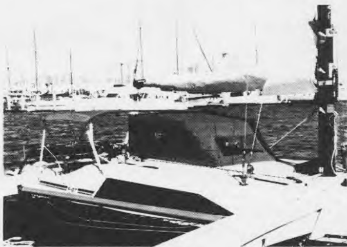
The Pop-top cover has been added here, for fully enclosed standing headroom while overnighting.
