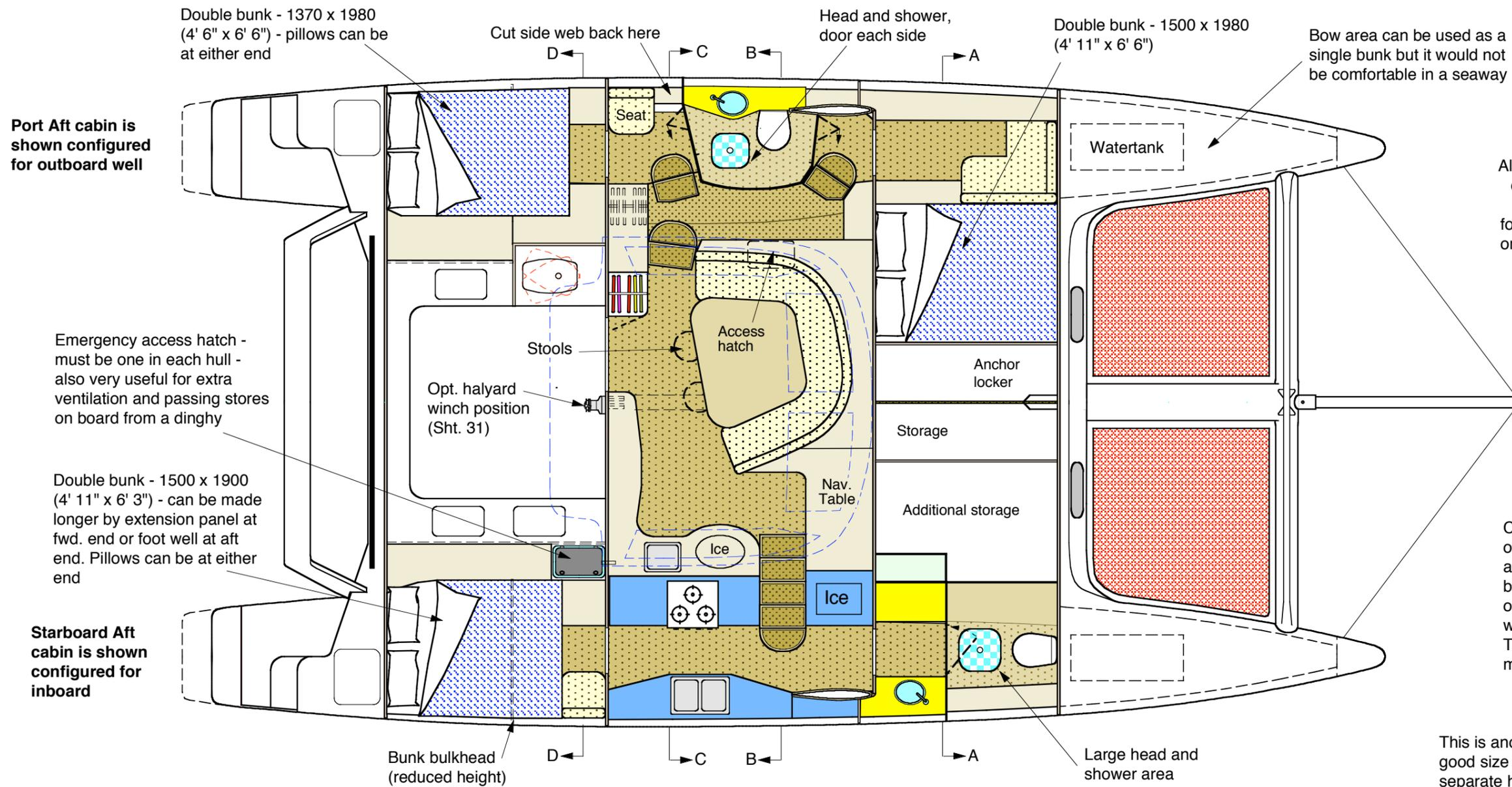
All cabin areas must have at least two exit routes. Forward cabins should thus be able to easily access the foredeck hatch via the inner hull side, or the optional bow hatch through the forward bulkhead.
